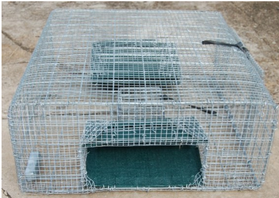
Figure 2. Fine mesh research pot with shade-cloth funnel
